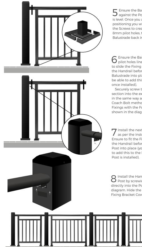
Ensure the Balustrade is secured old O against the Post, making sure it is level. Once you are happy with the positioning you will need to mark out the Screws to create pilot holes. Predrill 8mm pilot holes, then place the Balustrade back in place.
