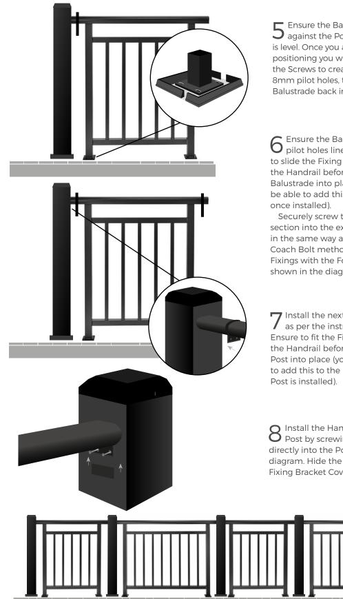
**5** Ensure the Balustrade is secured against the Post, making sure it is level. Once you are happy with the positioning you will need to mark out the Screws to create pilot holes. Predrill 8mm pilot holes, then place the Balustrade back in place.
