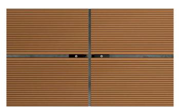
Where two Bamboo Board ends 6 meet (butt joints), each Board must be 2mm apart from each other and Fixing Clips must hold each Board into place at the meeting point.
