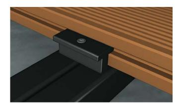
5 To install the next of your Boards, slide it onto your Fixing Clips securing the first Bamboo Board and fit an additional Fixing Clip set which will secure the adverse side of your Board, use a single Fixing Clip to every supporting Joist. With similar steps, fix the remaining Decking Boards. Board ends must be adequately supported. It is recommended to not have a overhang or cantilever.
