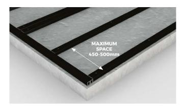
The Boards should not be placed directly onto the ground, they need to be fixed on the Joists. Between rows of Joists, the **recommended** space is 450-500mm. Double Joists are required where there are two Boards that meet at the ends. Screw Composite Joists into your concrete base.
