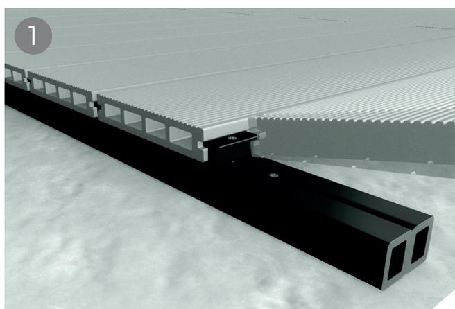
Step 1, after the last board of the main project has been laid, screw in a T clip along the edge of the final board. The bullnose board can then be inserted next to it.
