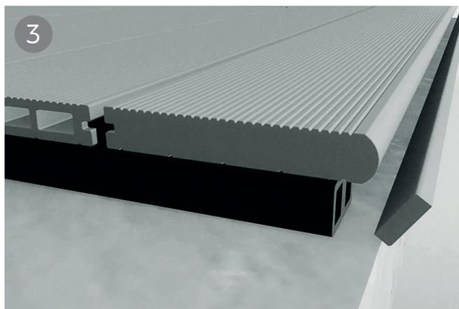
Step 3, once the bullnose board has been secured into place you can use a skirting board to neaten the edge. For higher areas you may wish to use a decking board as an edge.
