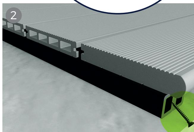
Step 2, once the bullnose board is placed you will need to insert a screw at an angle through the supporting joist underneath the board. Ensure the bullnose board is supported along the length with joists and a screw is inserted into each one.
