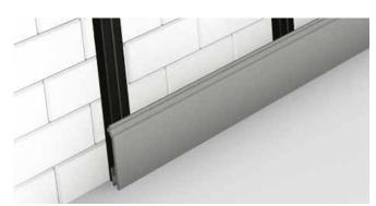
Secure the boards using a screw at least 20mm in length, ensuring that the board is fastened securely on each Joist that it touches. Secure these fixings by hand, is important not to over-tighten the screws and risk splitting the board. Ensure that the section between the Joists remains empty allowing air to flow beneath the boards.
