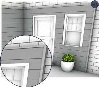
Installing the Corner Trims is the last phase of the project. Install the Composite Wall Cladding as above right up to any windows or doors.
