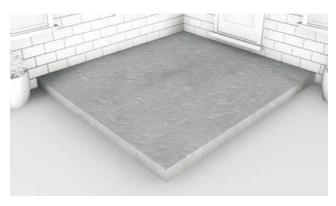
Make sure that the area to be decked is flat and stable. The concrete base should be at least 10cm thick and have a slight slope - we suggest a gradient of 1 in 80 - that runs away from the property to allow for the run-off of water that collects under the deck.
