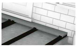
Our Composite Boards are easily fastened to the Joists of a supporting substructure with the help of our Stainless Steel Screw and plastic T-Clip System. Start at the outside of the area to be decked. Place your first board and fix it to each Joist it crosses using a row of Starter Clips.
