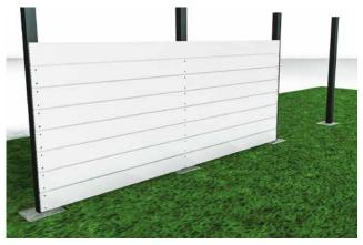
As you start to add more boards ensure each As you start to add more 222 fence panel is 100% level before fixing. Each Fence Panel slots on top of the board previously fitted. (Example shows 3.6m fence panels with Fence Post in between).
