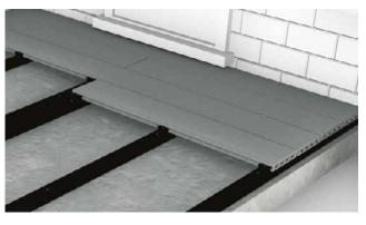
Fit your next board by sliding it onto the T-Clips used to secure the first board and fitting another set of T-Clips to secure the opposite side of the board, again one T-Clip for each supporting Joist. Follow a similar process to fix subsequent boards. The ends of boards must be fully supported. No overhang or cantilever is advised.
