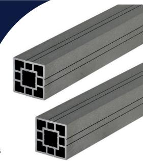
\*Please note: due to variations within the manufacturing process of these Posts, we advise to measure 20mm and channel this out rather than using the lines on the Posts, if installing Panels using the slot between method. If installing by securing to the front of the Composite Post, this process does not need to be followed.
