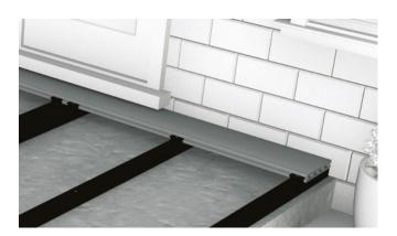
4 Our Composite Boards are easily fastened to the Joists of a supporting substructure with the help of our Stainless Steel Screws and plastic T-Clip System. Start at the outside of the area to be decked. Place your first Board and fix it to each Joist it crosses using a row of Starter Clips.
