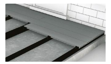
6 Fit your next Board by sliding it onto the T-Clips used to secure the first Board and fitting another set of T-Clips to secure the opposite side of the Board, using one T-Clip for each supporting Joist. Follow a similar process to fix subsequent Boards. The ends of Boards must be fully supported. No overhang or cantilever is advised.
