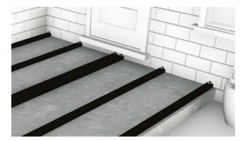
A Starter Clip needs to be fixed to the end of the Composite Joists before laying the first Board. Place these at the end of each Joist where you will start to lay your Boards, leaving a gap of 15mm between the wall and the end of the Joist to allow for expansion.
