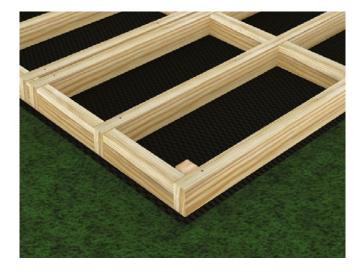
The maximum recommended space between Joist rows depends on the angle at which you intend to lay your boards in relation to the Joists, but should **never exceed 40cm**, please see diagram.
