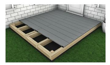
T Having fastened your Boards, all that remains is to tidy up the sides of your new Deck with our Composite Skirting or Fascia Boards, which can be used to hide the unfinished ends of Boards and supporting Joists.
