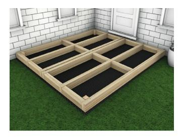
2 Starter Clips need to be fixed to the end of the Joists before laying the first Board. Place these at the end of each Joist, leaving a gap of 15mm between the wall and the Starter Clip to allow for expansion.
