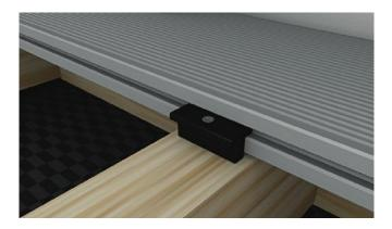
4 Slot T-Clips into the groove along the side of the Board and screw them into the supporting Joists with the screws provided, using one T-Clip for each supporting Joist. We recommend you use our Stainless Steel Wood Screws offering increased wear and less corrosion. **T-Clips will leave a 7mm gap between Boards.**
