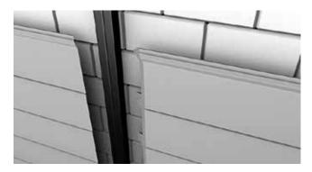
6 When butting two boards together, you should use a mitered edge for a neat finish. The most common miter angle is 45 degrees. As the cuts are angled, you'll have one side of the wood longer than the other. You'll need to keep track of which side will be which and make your measurements correctly.
