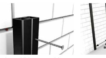
**1** You will need to pre-drill the Battens and the surface below using a 6mm drill bit, the Battens are 30mm high and you will need to secure them at least 50mm into the surface below. You will need to choose fixings suitable for the surface you are fixing into. Screws should be 5-6mm diameter and at least 80mm long\*.
