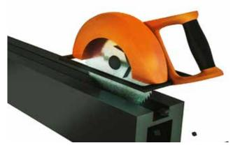
6 Alternatively you can fit the boards by slotting them into the Fence Posts. Cut up to four channels per post using the grooves as a guide. Then simply slide the Fence Board into the grooves.
