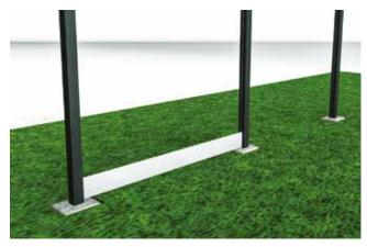
T When using the cut method the Fence Panels need to be cut into 1.6 metre lengths. The posts must be no further apart than 1.6 metres.
