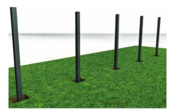
Prepare your area by removing any stones, debris or hazardous material. Dig the Fence Post Holes to 25% of the post height. The Fence Posts must be a maximum of 1.6m apart to ensure they can support the Fence Panels.
