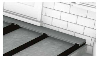
**5** Our Composite Boards are easily fastened to the Joists of a supporting substructure with the help of our Stainless Steel Screw and plastic T-Clip System. Start at the outside of the area to be decked. Place your first board and fix it to each Joist it crosses using a row of Starter Clips.
