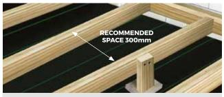
300mm joist spacings are recommended, you should never exceed 400mm spacings.
