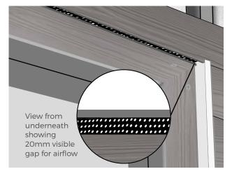
**STEP 4** Measure and cut the Fibre Cement Board in the same way as before and secure the Fibre Cement Board in place using 38mm Screws. Make sure there is at least a 20mm gap between the edge of the Board and the Perforated Trim to allow for adequate airflow.
