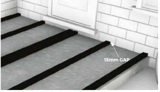
**3** A gap of at least 15mm should be left between the ends of Joists and a fixed object such as a wall and of at least 8mm between the ends of Joists at butt joints. These allow for proper drainage and temperature expansion.
