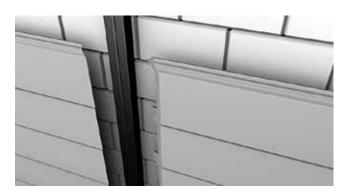
6 When butting two boards together, you should use a mitered edge for a neat finish. The most common miter angle is 45 degrees. As the cuts are angled, you'll have one side of the wood longer than the other. You'll need to keep track of which side will be which and make your measurements correctly.
