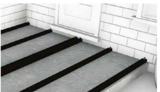
4 A Starter Clip needs to be fixed to the end of the composite Joists before laying the first board. Place these at the end of each Joist where you will start to lay your Boards, leaving a gap of 15mm between the wall and the end of the Joist to allow for expansion.
