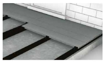
**7** Fit your next board by sliding it onto the T-Clips used to secure the first board and fitting another set of T-Clips to secure the opposite side of the board, again one T-Clip for each supporting Joist. Follow a similar process to fix subsequent boards. The ends of boards must be fully supported. No overhang or cantilever is advised.
