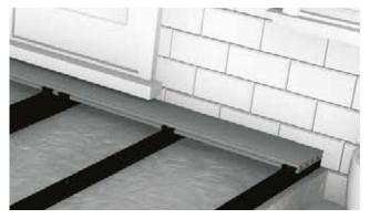
**5** Our Composite Boards are easily fastened to the Joists of a supporting substructure with the help of our Stainless Steel Screw and plastic T-Clip System. Start at the outside of the area to be decked. Place your first board and fix it to each Joist it crosses using a row of Starter Clips.
