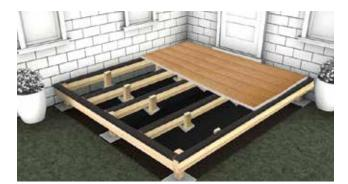
T Start by laying out your Decking Boards onto the desired area before fixing them in place. Ensure there is a 3mm gap between any boards at butt ends or side by side and between all walls and fences.
