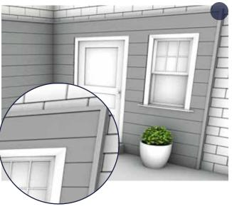
Installing the Corner Trims is the last phase of the project. Install the Composite Wall Cladding as above right up to any windows or doors.
