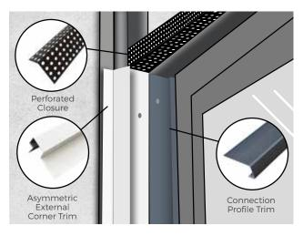
**STEP 1** Alongside the Asymmetric External Corner Trims previously installed around windows and doors, secure Connection Profile Trims to the internal corners of a window or door reveal using 38mm Screws, as shown in the diagram. Make sure that the small painted edge of the Connection Profile Trim sits neatly against the window or door frame.
