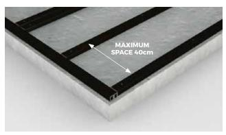
2 Boards must not be laid directly on the ground but should be fixed to the Joists. The maximum recommended space between Joist rows depends on the angle at which you intend to lay your Boards in relation to the Joists, but should **never exceed 40cm**, please see diagram (above). Composite Joists should be screwed into the concrete base.
