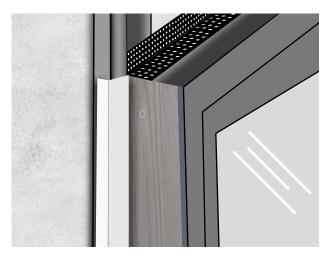
**STEP 2** Cladco Fibre Cement Boards can be cut to the same width as the window or door reveals using a wet saw and a Level P3 Respiratory Protective Mask. Slot the Board between the Connection Profile Trim and the Asymmetric External Corner Trim. Use 38mm Screws to fix the Boards into place.
