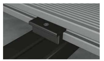
6 Then fit T-Clips into the groove along the side of the board and screw them into the supporting Joists with the screws provided, one T-Clip for each supporting Joist. We recommend you use our Stainless Steel Wood Screws offering increased wear and less corrosion. T-Clips will leave a 7mm gap between boards.
