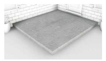
Make sure that the area to be decked is flat and stable. The concrete base should be at least **10cm thick** and have a slight slope - we suggest **a gradient of 1 in 80** - that runs away from the property to allow for the run-off of water that collects under the deck.
