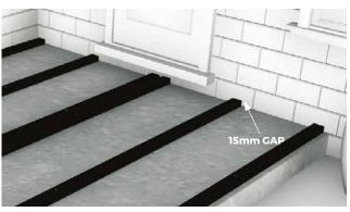
**3** A gap of at least 15mm should be left between the ends of Joists and a fixed object such as a wall and of at least 8mm between the ends of Joists at butt joints. These allow for proper drainage and temperature expansion.
