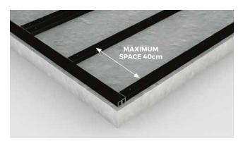
Boards must not be laid directly on the ground but should be fixed to the Joists. The maximum recommended space between Joist rows depends on the angle at which you intend to lay your Boards in relation to the Joists, but should **never exceed 40cm**, please see diagram (above). Composite Joists should be screwed into the concrete base.
