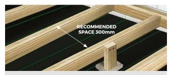
300mm joist spacings are recommended, you should never exceed 400mm spacings.
