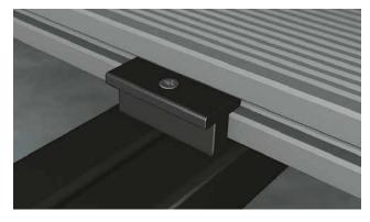
Then fit T-Clips into the groove along the side of the board and screw them into the supporting Joists with the screws provided, one T-Clip for each supporting Joist. We recommend you use our Stainless Steel Wood Screws offering increased wear and less corrosion. T-Clips will leave a 7mm gap between boards.
