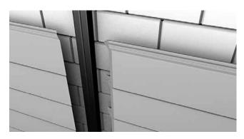
When butting two boards together, you should 6 use a mitered edge for a neat finish. The most common miter angle is 45 degrees. As the cuts are angled, you'll have one side of the wood longer than the other. You'll need to keep track of which side will be which and make your measurements correctly.
