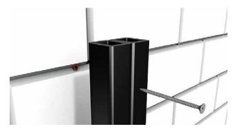
You will need to pre-drill the Battens and the surface below using a 6mm drill bit, the Battens are 30mm high and you will need to secure them at least 50mm into the surface below. You will need to choose fixings suitable for the surface you are fixing into. Screws should be 5-6mm diameter and at least 80mm long\*.
