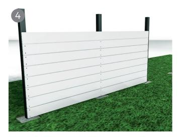
As you start to add more boards ensure each fence panel is 100% level before fixing. Each fence panel slots on top of the board previously fitted. (Example shows 4m fence panels with fence post in between).
