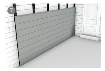
Continuing to fit the cladding boards in this manner until you have completely covered the area you want. It is possible to fit your boards side by side simply but the two ends up together. You may need to install more battens if you wish to do this as each board will need to be supported on a joist where it meets the next board.
