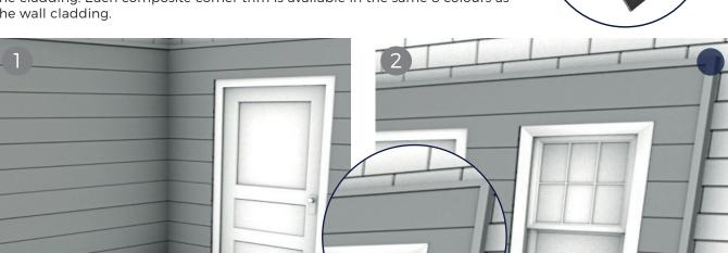
Installing the corner trims is the last phase of the project, install the composite wall cladding as above right up to any windows or doors.
