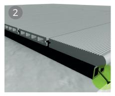
Once the bullnose board is placed you will need to insert a screw at an angle through the supporting joist underneath the board. Ensure the bullnose board is supported along the length with joists and a screw is inserted into each one.
