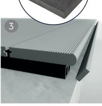
Once the bullnose board has been secured into place you can use a skirting board to neaten the edge. For higher areas you may wish to use a decking board as an edge. Secure the skirting edge with either a screw into each joist or using sumo grip adhesive.
