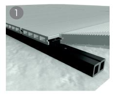
After the last board of the main project has been laid, screw in a T clip along the edge of the final board. The bullnose board can then be inserted next to it.
