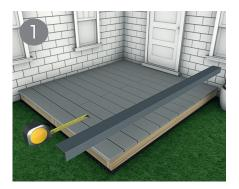
Take the corner trim and measure the length of the area its going to be fitted on to. Corner trims can be cut and worked just like timber so can be cut to desired size. If placing two trims side by side, simply butt up together.
