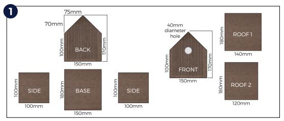
Cut the decking into the required lengths as shown above. Take care if using hollow decking as the honeycomb structure may split. Cutting the edges may create sharp sides so care should always be taken.
