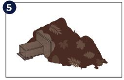
Line the inside of the house with newspaper, dry leaves, and straw. Cover with polythene sheeting (optional). Pack soil and dead leaves around the outside of the house, being careful to keep the entrance pip and ventilation holes free of debris.
