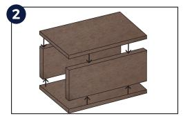
Using sumo grip adhesive, glue the four pieces of composite decking into a tunnel shape. If you don't have adhesive you can use screws instead, but be careful to not split the boards. If you're using sumo grip adhesive, it is advisable to place a heavy object on top of the seal and leave the glue to dry for at least 24 hours.
