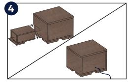
Attach the tunnel, the tunnel will be slightly shorter than the height of the opening, this can then be slotted in at a slight angle, creating a ramp. For extra ventilation, drill a small hole in the back of the box and fit part of a hosepipe in.
