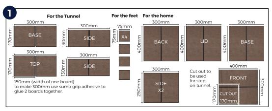
Our decking boards are 150mm wide, for the desired size of the hedgehog house please glue/cut your excess boards to the sizes shown. Take care if using hollow decking as the honeycomb structure may split. Cutting the edges may create sharp sides so care should always be taken.
