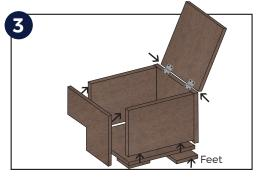
Use one of the 400mm x 300mm boards as the hedgehog house lid. Attach the two metal hinges to the side of the lid.
