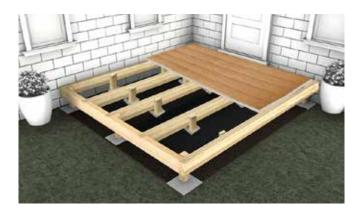
Start by laying out your decking boards onto the desired area before fixing them in place. Ensure there is a 3mm gap between any boards at butt ends or side by side and between all walls and fences.
