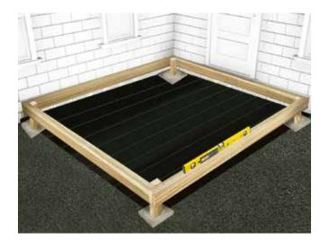
J If your deck will be sitting on grass or soil, you will need to place blocks or slabs underneath each leg, to spread the load and provide a level, stable base. Additional blocks can be used if required. Position and adjust the blocks/slabs, ensuring the frame is at a slight angle, that will allow the water to drain down the length. We recommend a slope of at least 5mm for every meter. Alternatively, if using slabs, you could dig a hole and set the legs in concrete.
