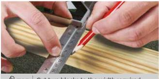
TOP<br/>TIPCut two blocks to the width required<br/>and use this as spacers for the joists.
