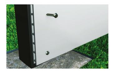
Alternatively, each 3.6m Panel can be secured to the front of the Post, with a supporting Post every 1.8m behind to provide stability. When adding the first Fence Panel, ensure it is 100% level before fixing to Posts. Screw the top and bottom of each Fence Panel to the Fence Posts behind.
