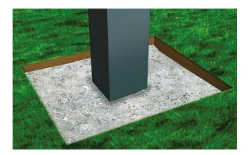
Make sure every Fence Post is 100% level before using postcrete. Fence Posts must have at least 25% of their height concreted into place.
