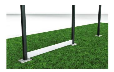
When using the slot between method, Fence Panels need to be cut into 1.8m lengths. Posts must be 1.8m apart and include an extra 5mm gap each end to allow for expansion of the Panels.
