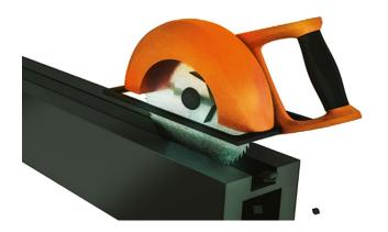
If using the slot between method, cut up to four channels per Post. Please ensure you leave an adequate expansion gap when using the slot in method to allow for natural expansion of the Panels.
