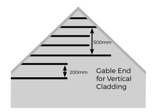
If your home has a gable end, Battens must be spaced up to 500mm apart with additional, shorter supporting Battens installed every 200mm, going up and down the apex (the triangular shape of your gable end). This ensures that the Composite Boards are fully supported across the entire build.
