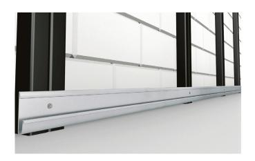
Attach a Starter Strip to the bottom of each Batten. This will give the first Cladding Board something to sit on. You will need to pre-drill a pilot hole into the Composite Batten and attach the Starter Strip using a screw that is at least 15mm long. Ensure that each Strip is level with the next and that the first Board sits level on the Strips before continuing to the next step.
