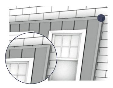
Once the Corner Trim is cut to size, you can use Sumogrip adhesive along one or both sides of the Corner Trim to attach it to the edge of the Cladding.
