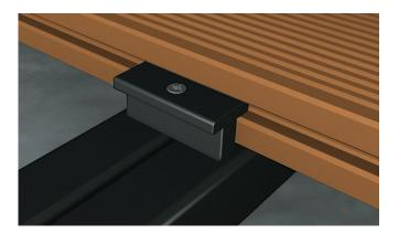
**5** To install the next of your Boards, slide it onto your Fixing Clips securing the first Bamboo Board and fit an additional Fixing Clip set which will secure the adverse side of your Board, use a single Fixing Clip to every supporting Joist. With similar steps, fix the remaining Decking Boards. Board ends must be adequately supported. It is recommended to not have a
