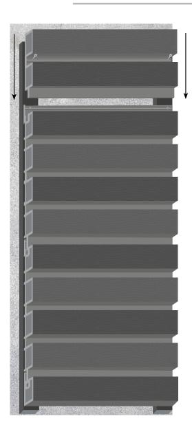
top of the first using the tongue and groove method. The non-grooved lip of the second panel will conceal the screws from the first and secured on the top grooved lip. Repeat this process with each Slatted Panel until you reach the required height and coverage, making sure that each panel is securely fixed to the Batten underneath.
