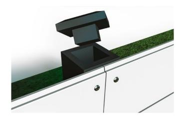
**7** Once the desired height has been reached (no more than 2.25m or 10 Panels) simply place the Composite Fence Cap on top of the Post. These are also available in all eight colours to match your Composite Fence. Fence Post Caps simply sit on top of the Post and do not need to be secured.
