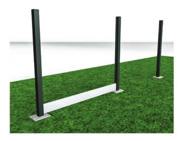
When using the slot between method, Fence Panels need to be cut into 1.8m lengths. Posts must be 1.8m apart and include an extra 5mm gap each end to allow for expansion of the Panels.
