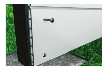
Alternatively, each 3.6m Panel can be secured to the front of the Post, with a supporting Post every 1.8m behind to provide stability. When adding the first Fence Panel, ensure it is 100% level before fixing to Posts. Screw the top and bottom of each Fence Panel to the Fence Posts behind.
