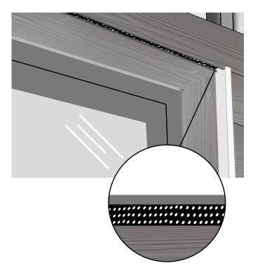
View from underneath showing 20mm visible gap for airflow
