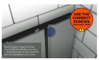
Ensure that the section between the Battens remains empty allowing air to flow beneath the Boards. Slot the second Board onto the first and repeat the fixing process ensuring that the second Board is fitted securely in place on each Batten.
