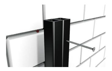
You will need to pre-drill the Battens and the surface below using a 6mm drill bit. The Battens are 30mm high and you will need to secure them at least 50mm into the surface below. You will need to choose fixings suitable for the surface you are fixing into. Screws should be 5-6mm diameter and at least 80mm long\*.
