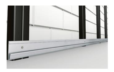
Attach a Starter Strip to the bottom of each Batten, leaving a 10mm ventilation gap at the base of the installation. Ensure no sealant is applied around this area. This will give the first Cladding Board something to sit on. You will need to pre-drill a pilot hole into the Composite Batten and attach the Starter Strip using a screw that is at least 15mm long. Ensure that each Strip is level with the next and that the first Board sits level on the Strips before continuing to the next step.
