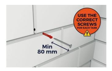
You will need to pre-drill the Battens and the surface below using a 6mm drill bit. Cladco Composite Battens are 30mm high and you will need to secure them at least 50mm into the surface below. You will need to choose fixings suitable for the surface you are fixing into. Screws should be 5-6mm diameter and at least 80mm lona\*.
