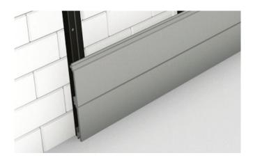
Slot the second Board onto the irst and repeat the fixing process ensuring that the second Board is fitted securely in place on each Batten. Repeat this process with each Board until you reach the required height. Ensure that the section between the Battens remains empty to allow air to flow beneath the Boards.
