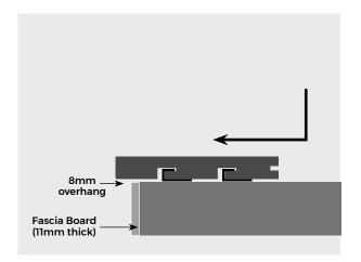
Fit the ProDeck Bullnose Composite Decking Board over the starter/bullnose clips and push forward until flush. Secure in place with T-clips as required before continuing to fit the rest of your standard ProDeck Composite Decking Boards.
