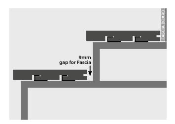
Install the ProDeck Bullnose Composite Decking Board as above on each step, leaving a small 9mm gap behind to allow the fascia trim to fit. Fit the fascia trims on each step to conceal the decking underneath. Ensure you have planned and measured your steps in accordance with the bullnose board's and fascia trim's dimensions to avoid any vacant space.
