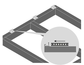
Bullnose boards/starter clips need to be fixed to the end of the joists before laying the first board, leaving a gap of at least 10mm between any walls and the starter clip. Use one bullnose/starter clip and screw per joist. Place the first ProDeck Composite Decking Board on the timber frame, ensuring the boards run perpendicular to the joists and secure the first board into the first bullnose/starter clips. Do not screw through the ProDeck Composite Decking Board.
