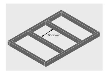
The maximum recommended space between recycled plastic joist rows depends on the angle at which you intend to lay your boards about the joists, but should never exceed 300mm (please see the diagram). If using timber joists, apply deck tape to the top surface and exposed cut ends to protect them from moisture and prevent rotting.
