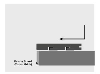
Tit the bullnose board over the starter/ bullnose clips and push forward until flush. Secure in place with T-clips as required before continuing to fit the rest of your standard ProDeck Composite Decking Boards.
