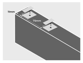
Using the same timber frame substructure, fit two ProDeck Bullnose/Starter Clips to the end of your joists as shown here, ensuring they are spaced 75mm apart with the first clip being 11mm from the edge joist.
