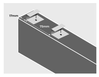
Using the same substructure, fit two ProDeck Bullnose/Starter Clips to the end of your joists as shown here, ensuring they are spaced 75mm apart with the first clip being 17mm from the edge of the joist.
