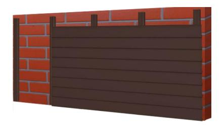
Slot the second board onto the first and repeat the fixing process ensuring that the second board is fitted securely in place on each joist.
